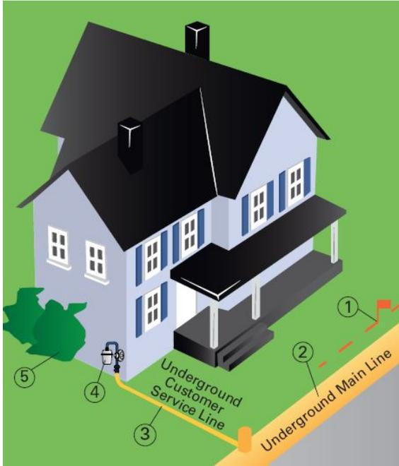
1. **MARK** the right of way and existing utilities with flags, stakes, and temporary paint. When we make personal contact with you, please alert us to any sprinkler systems or invisible dog fences.
